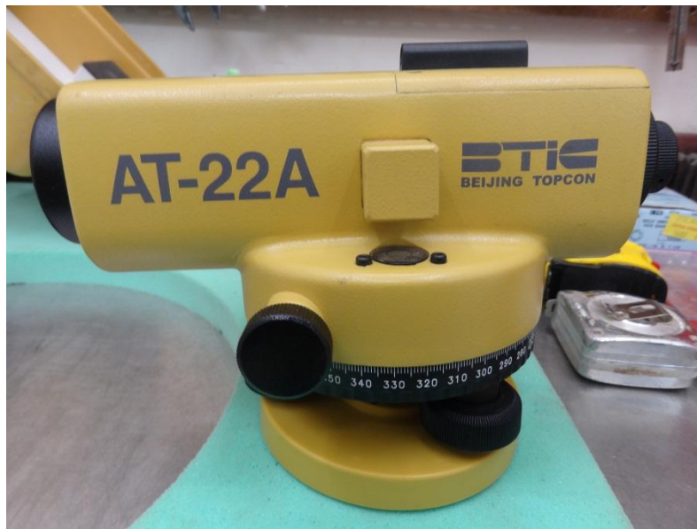
Figure 19. Level for measuring the road profile
